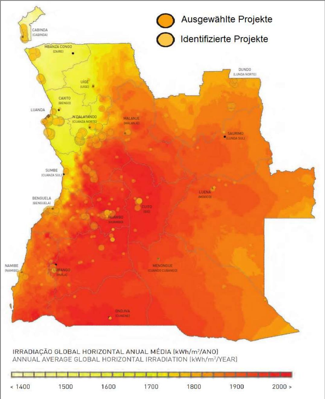
**Figure 4: Solar resources, identified and selected projects to achieve the 100 MW target (Ministério de Energia e Águas de Angola, n.d.)**
