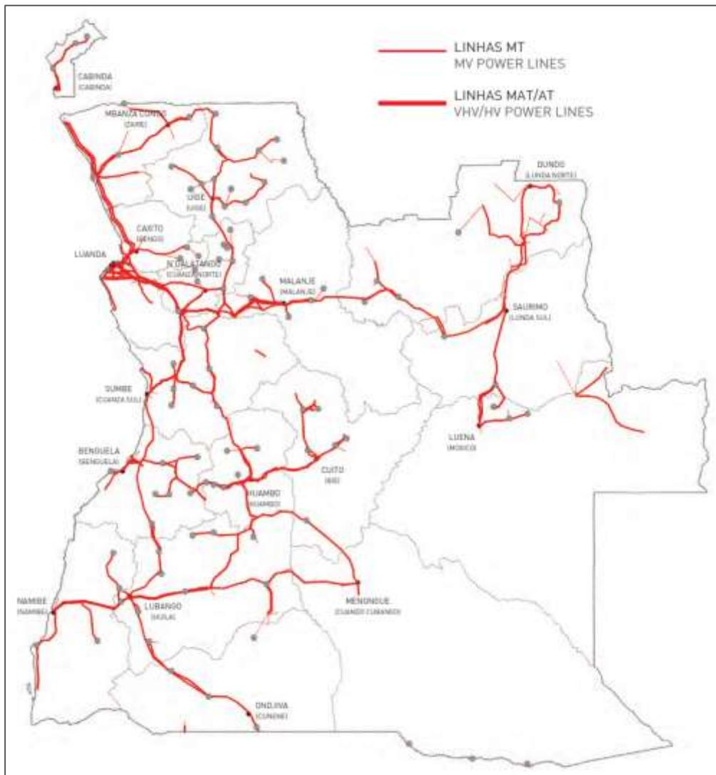
**Figure 5: Electrification of communities outside large urban areas through the expansion of the national electricity distribution grid (Ministério de Energia e Águas de Angola, n.d.).**
